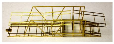
There are two sizes of Adjustable Ramps, long and short. VERY IMPORTANT: One Short Ramp is slightly wider than the other. The wider Short Ramp is for the front of the Cab. Clean up two Long Ramps and one Short Ramp after removing from the kit. The exact placement is up to the builder, but a common configuration is shown for carrying vehicles. If the Carrier is to be modeled during loading, the Adjustable Ramps would be attached as a Ramp from the end to the Cab locations.
