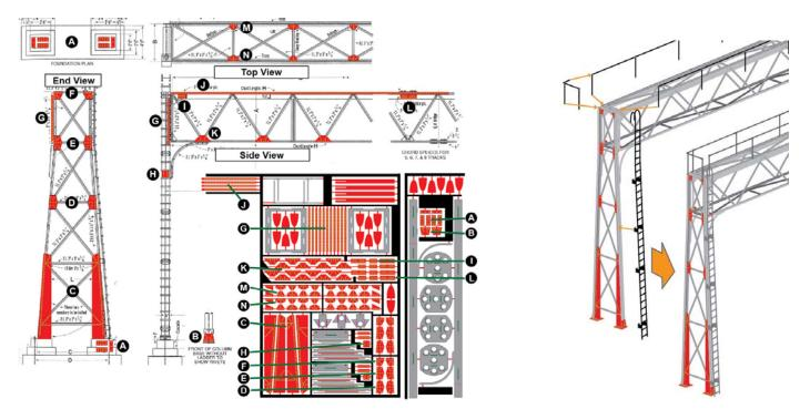
The builder should reference the image above to see where each of the Detail Overlays are to be placed onto the model. A locator is also shown to help the builder find the overlays on the kit sprue. It is advisable for the user to add the details by the alphabet. Detail C, D, F and F already had to be installed to properly build the End Bents.
