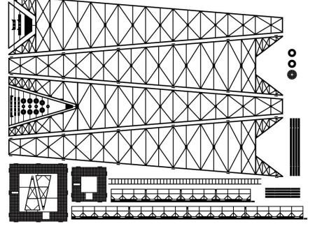
second cut to remove all of the ties, sometimes holding the part under a magnifying glass will help. This will reduce or eliminate the amount of filing to smooth the edge. The next best way is with small sharp diagonal cutters that will fit into the small areas between the part and the sheet holding them. *You should always use a file to remove the balance of the tie. This will ensure a perfect fit.*
