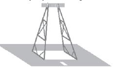
e) Attach the completed A-frame to the small platform. Be sure to orientate the A-frame to allow a cable to be threaded through the A-frame pulley and the pulley on the small platform.
