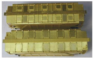
The kit includes four small triangular pieces that secured to the inside of the Sill to hold the Air Line which is made from the provided ,.010" wire. Secure the Supports to the Sill and then the Air Line to the Supports.
