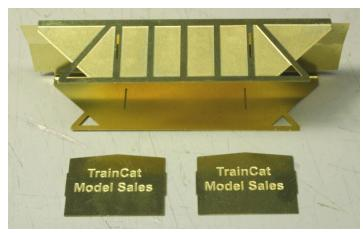
Install the Body Forms into Shell from underneath. Each Body Form has tabs on it's sides that fit into slots on the shell. Depending on how well you bent the sides, you may need to file the sharp edges at the top to fill the bend. Secure the Body Forms to the Shell.
