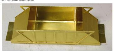
Using care, remove the two side Detail Overlays from the kit sprue and remove all tie remnants. This piece is thin and could be distorted if handled roughly. Add the Detail Overlay onto the Shell Sides over the raised portion.
