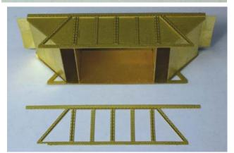
Place the Sell assembly top down. The builder should notice that there are two etched lines on the End Panels. These lines will aid in the placement of End Details and components. Remove the End Rivet Detail from the sprue. The smaller section of the Rivet Detail begins at the first etch line. The full width cross piece is aligned at the second etch line. The longer section continues down the middle, over the bend up to the Roof.
