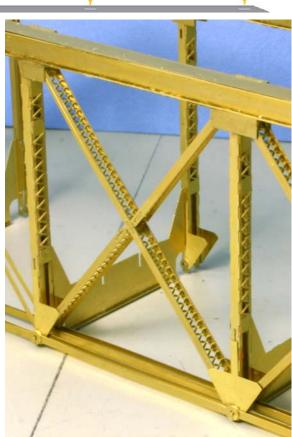
E) Apply the Splice Plate detail from short member to short member over the long member. This will cover-up any gaps in the joint.
