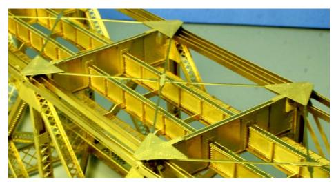
Repaeat for all Lower Lateral Braces. Please note that the Shoe Plate at the ends of the bridge is the place to attach the end Laterals.
