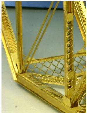
E) Using .032 rod cut to 1/2in lengths as pins, begin connecting the Main Eyebars to the Posts following the diagram. Do not secure, nor trim pins yet. Use a small piece of painters masking tape to keep Eyebars from removing themselves from the pins.
