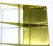
Secure the two end Joists to Roof Panel ensuring the tabs on the Peak Stringer go into the notches of the Joists.
