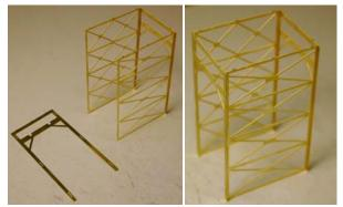
To build the Stair Support Column, remove the pieces shown from the kit fret and remove all tie remnants.
